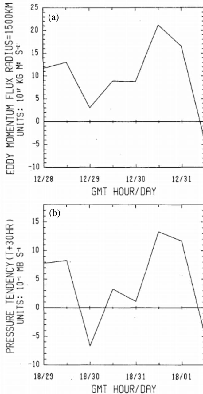
Fig. 1.5. (a) Eddy momentum flux at the 1500 km radius, plotted only for those times in which the storm remained over water 30 h later. (b) Deepening rate of the storm at times 30 h after those of part (a). Caption and figure reproduced from Fig. 4 in Molinari and Vollaro (1989).
