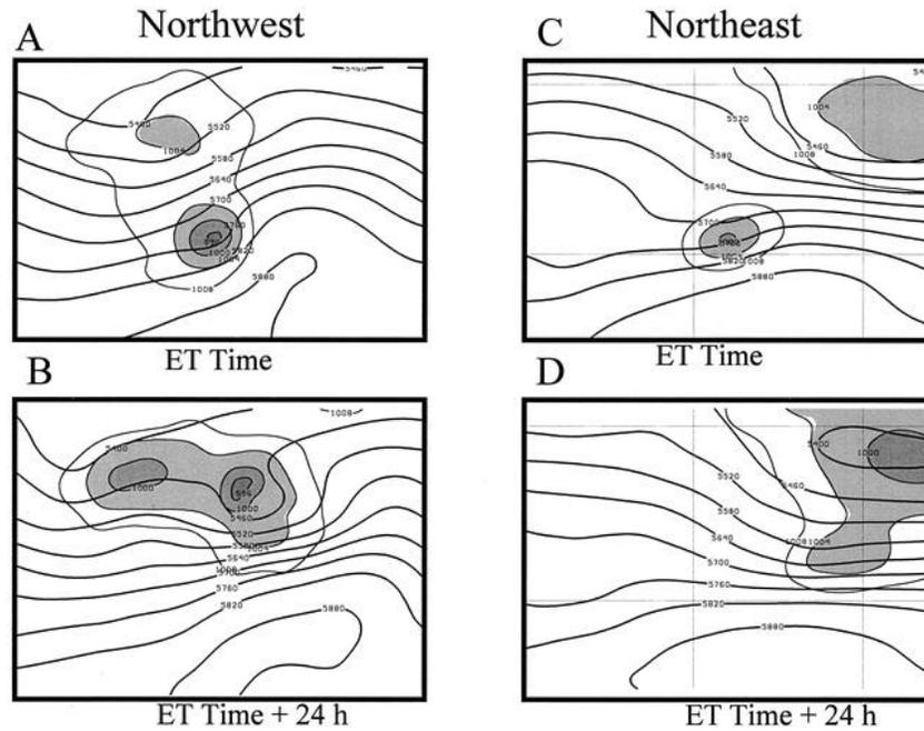
Fig. 1.2. Composite 500-hPa height (m) and sea level pressure (hPa, only below 1008 hPa with shading in 4-hPa increments starting at 1004 hPa) analyses based on grouping of cases in a northwest pattern at the (a) ET time, (b) ET + 24 h, and in a northeast pattern at the (c) ET time and (d) ET + 24 h. The composite northwest pattern is based on 13 cases and the northeast pattern is based in 17 cases. Caption and figure reproduced from Fig. 1 in Harr et al. (2000).
